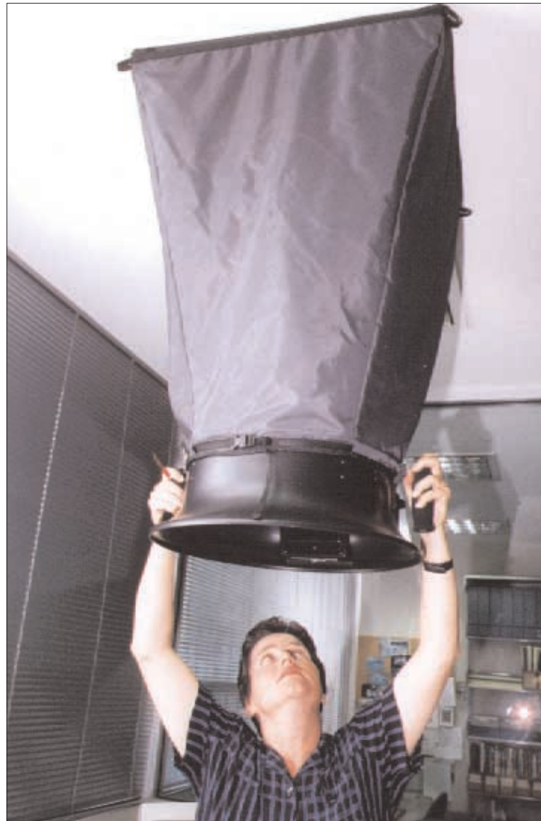
CSIRO now has facilities to calibrate flow hoods used in the air conditioning industry.
