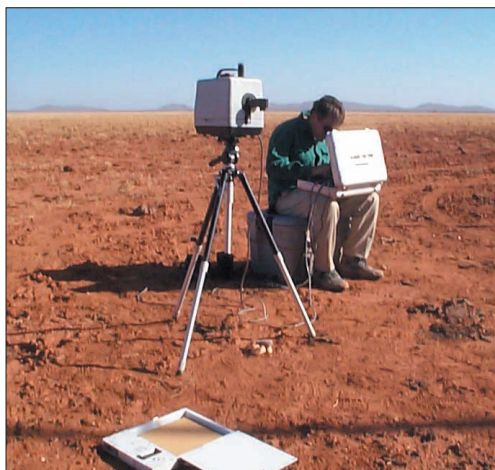
Dr Simon Hook, a NASA JPL scientist, makes radiometer measurements at Amburla in central Australia.
