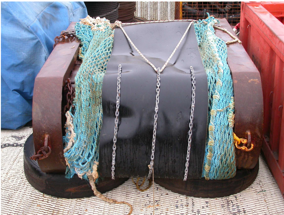
Figure 4: The conveyor belt and its attaching chains. Note the bolts in the chains and how far up the mat the chains run to spread the load. The mat is lashed up over the sled to give a better idea of how the chains are attached.
