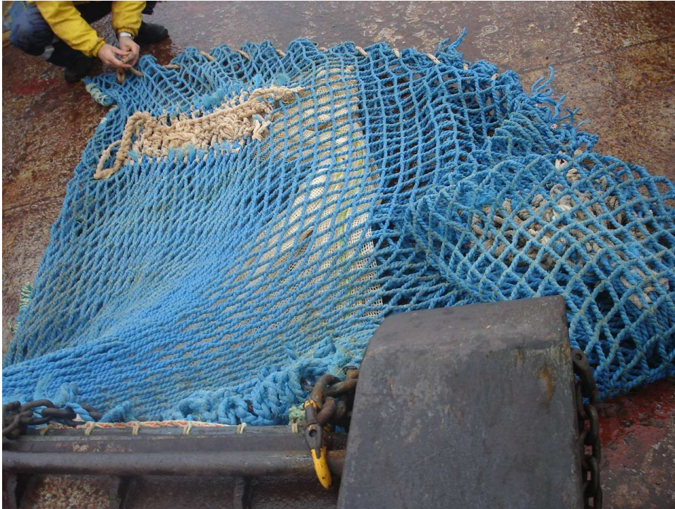
Figure 4: The conveyor belt and its attaching chains. Note the bolts in the chains and how far up the mat the chains run to spread the load. The mat is lashed up over the sled to give a better idea of how the chains are attached.
