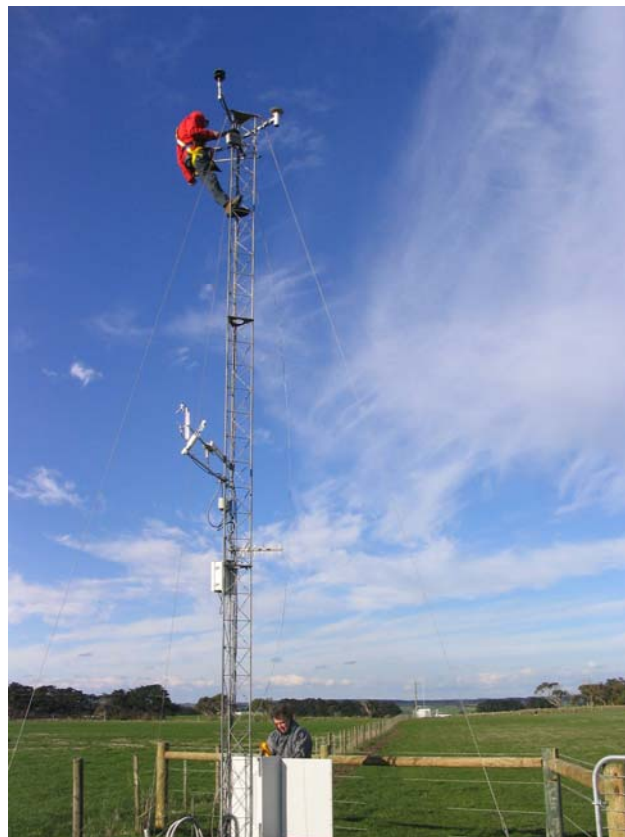
Figure 6. Setting up the flux station. The atmospheric module is in the distance.
