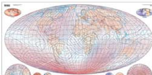
The International Geomagnetic Reference Field (IGRF) as published in a USGS chart. Red lines of equal intensity running approx. east-west establish a north-south gradient in many parts of the world. Magnetic field intensity measurement can readily determine latitude within tens of miles.
