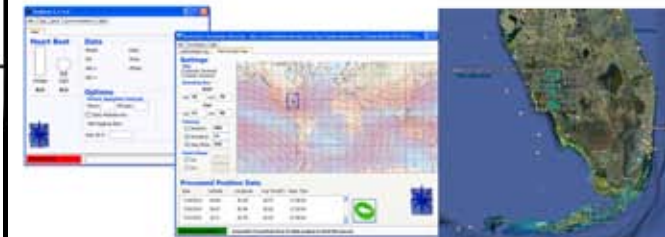
(left to right) SeaDock software is used to configure and download data to/from the tags. SeaTrack software (middle) is used to process the data from the tag. Several processing filters are included such as averaging over days, maximum distance traveled per day, and a magnetic offset. The data is then exported into a standard txt file or a Google Earth file for immediate viewing.
