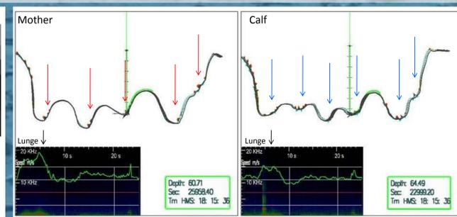
Dtags<sup>1</sup> were attached to a humpback whale mother and calf pair and logged 18 hours of concurrent recordings (11:55 am - 7:46 am). Depth, heading, pitch and roll were digitally recorded at 50 Hz and stored, synchronously, with audio data (sampling rate 96 kHz) on flash memory within the tag.
