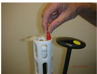
4) Carefully remove the black rubber plug from the bottom center of the yellow cowling as shown in the image below. This will allow you to verify air bladder inflation in the steps below. Use only your fingers to remove the plug. Tools may puncture or otherwise harm the bladder. Be sure to replace the plug before deployment!
