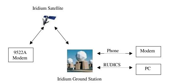
For modem-to-modem communications (without RUDICS) you will need independent primary and alternate host servers, each with a modem connected to the phone system to receive the calls and data from the float. A full description of this equipment and software is beyond the scope of this manual. However, Teledyne Webb Research makes regular use of U.S. Robotics external modems, Model USR3453C, Courier<sup>TM</sup> 56K Business Modem.
