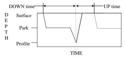
Parameter **PD** determines the frequency of deep profiles. Schematic examples:
